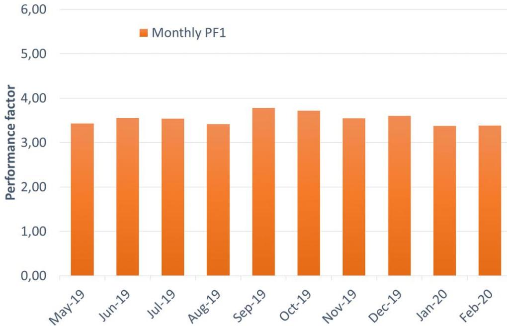
Figure 24. Monthly Performance Factor (MPF) of the heat pumps
