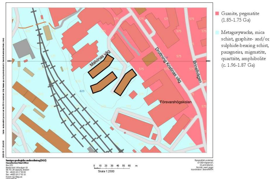
Figure 5. Local geological map around the Forskningen 2 site. Adapted from SGU.
